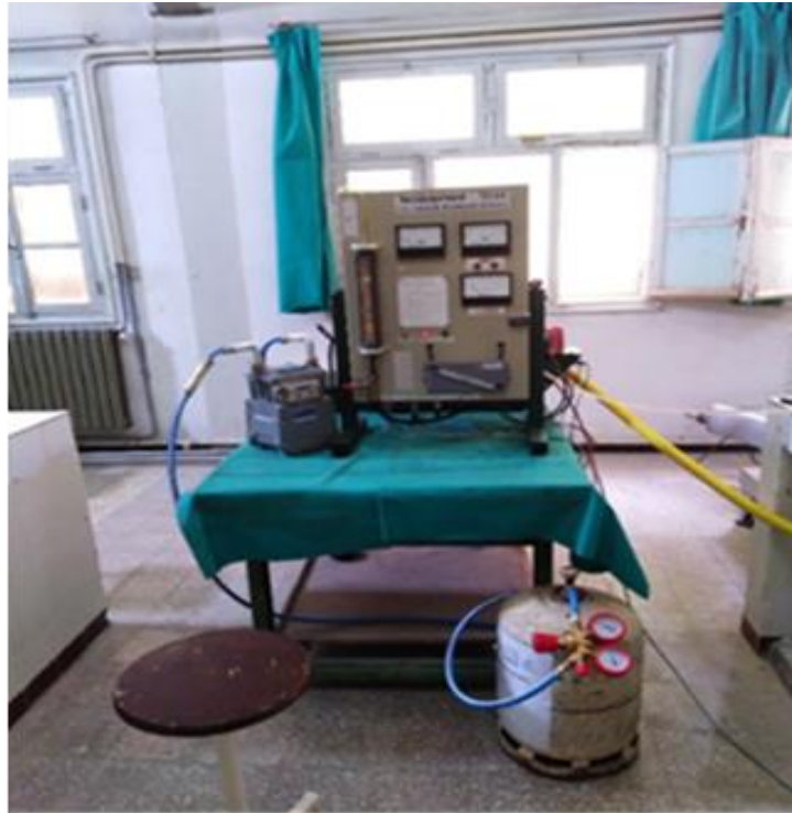
Figure 3-35 The test rig set-up runs on biogas[102]
