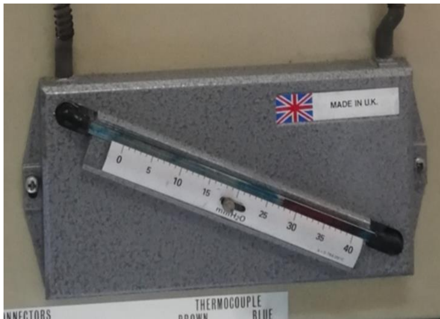
Figure 3-15 Inclined manometer for reading the pressure difference
