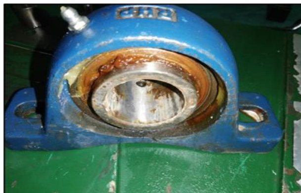
Figure 3-24 the bearing and oil seals changing.
