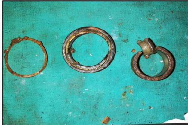
Figure 3-22 The broken oil seals and bearings
