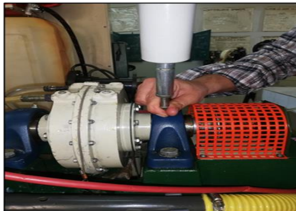
Figure 3-27 Lubricating of bearings
