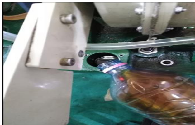
Figure 3-26 Oil damper tank adding
