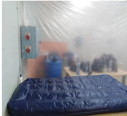
Figure 2-11 The biogas storage
