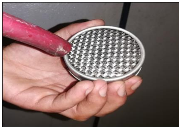
Figure 3-16 Air filter and air filter holder cleaning
