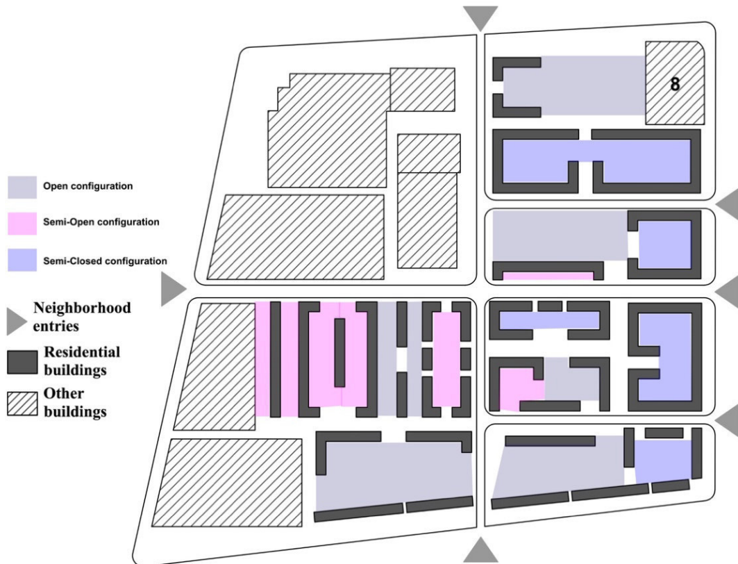
Figure 33 Different types of spatial configurations of the neighborhood of 420 housing units (Source: Author).
