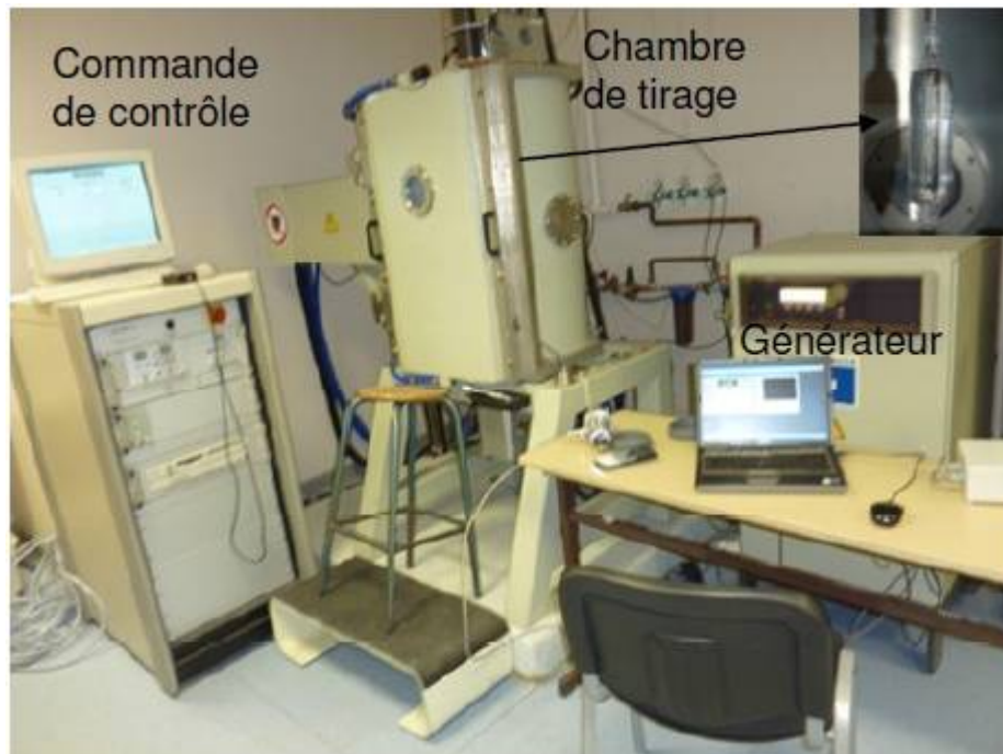
Figure II.20 : Machine de tirage Czochralski. Institut ILM. Lyon-France [7].
