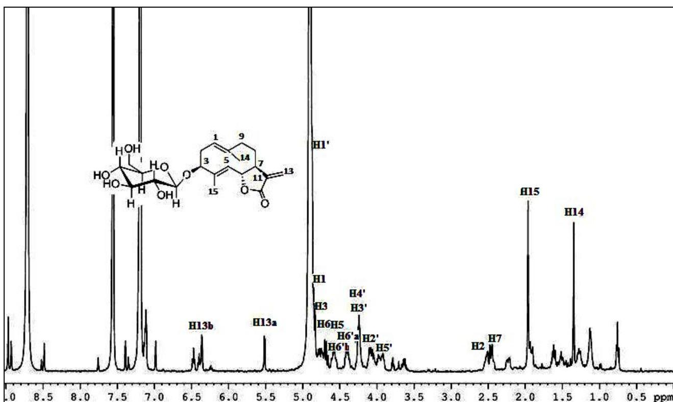
Figure 3.109:  $^1\text{H}$  NMR spectrum of compound **316** in  $\text{pyridine-}d_5$
