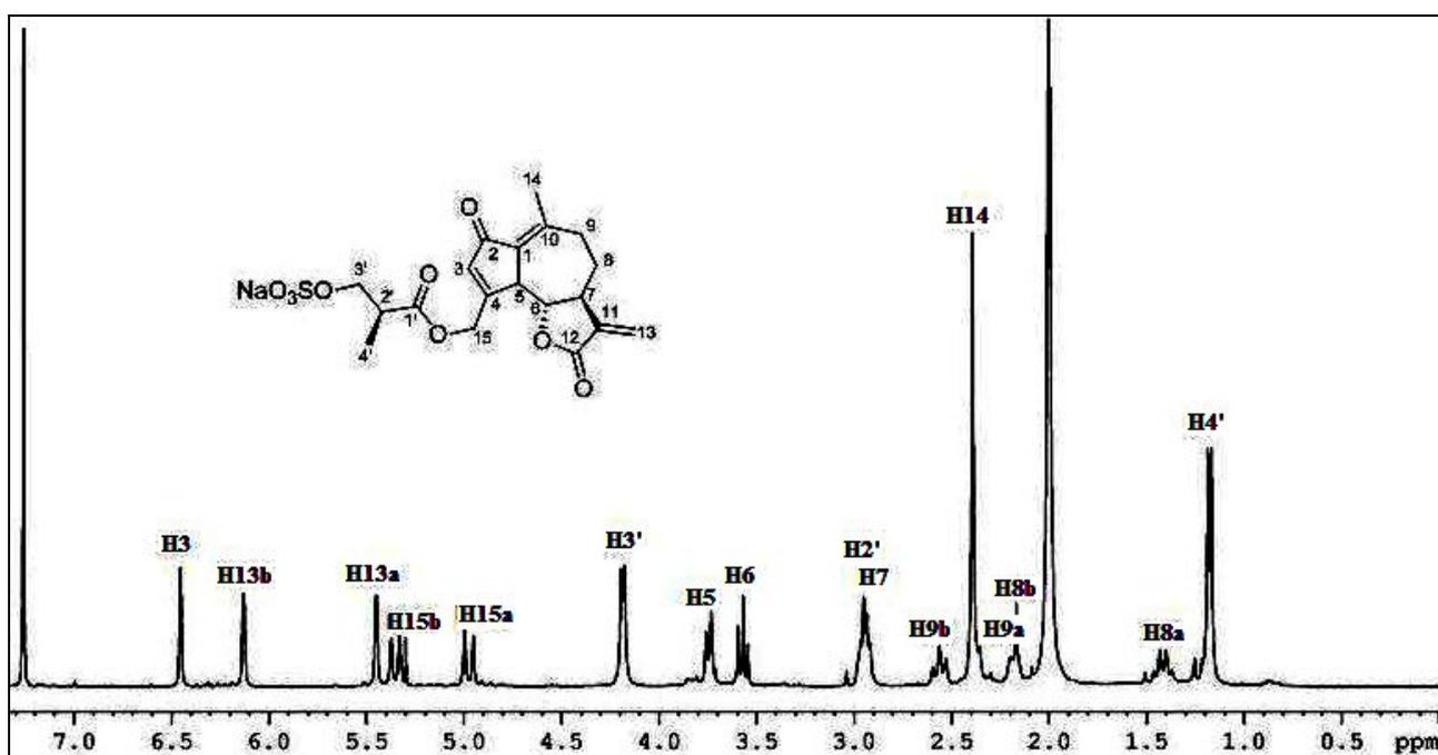
Figure 3.68:  $^1\text{H}$  NMR spectrum of the compound 311 in  $\text{CDCl}_3$
