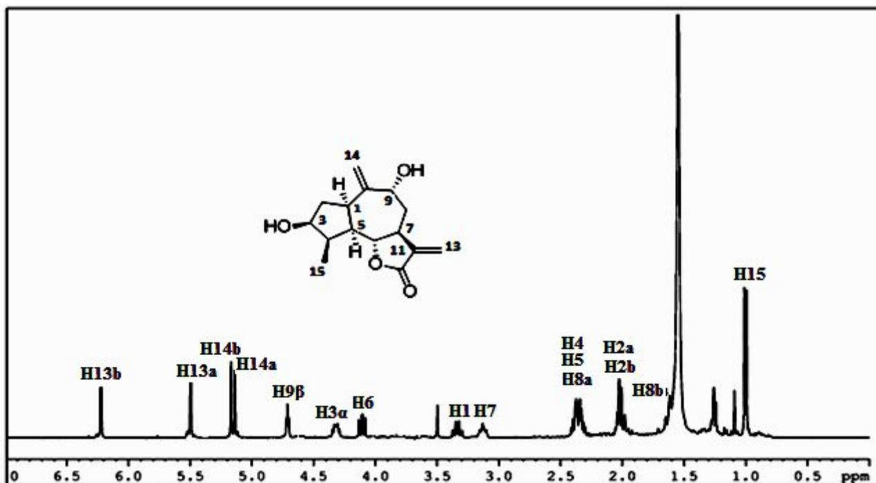
Figure 3.54:  $^1\text{H}$  NMR spectrum of the compound 306 in  $\text{CDCl}_3$
