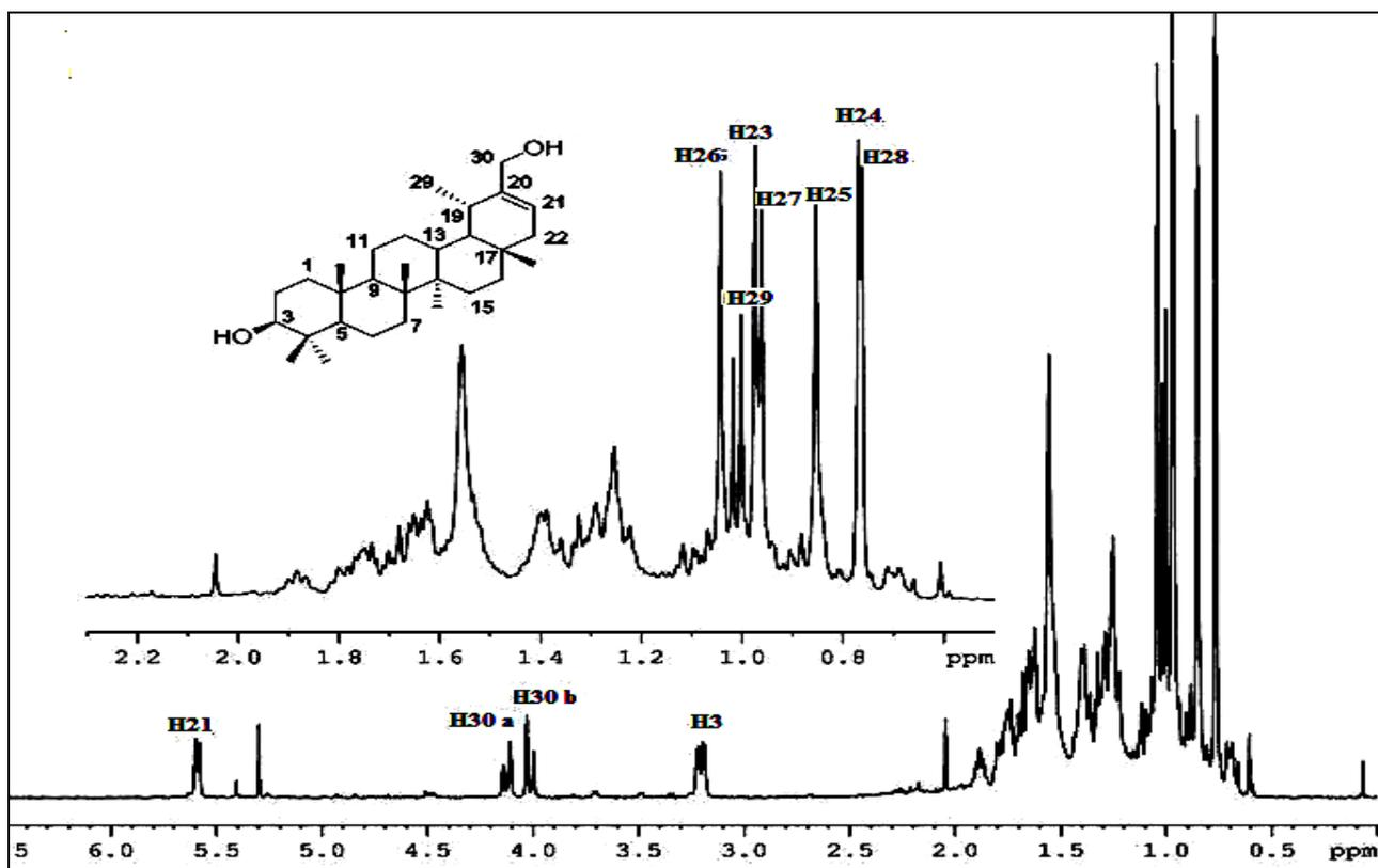
Figure 3.36:  $^1\text{H}$  NMR spectrum of compound **302** in  $\text{CDCl}_3$
