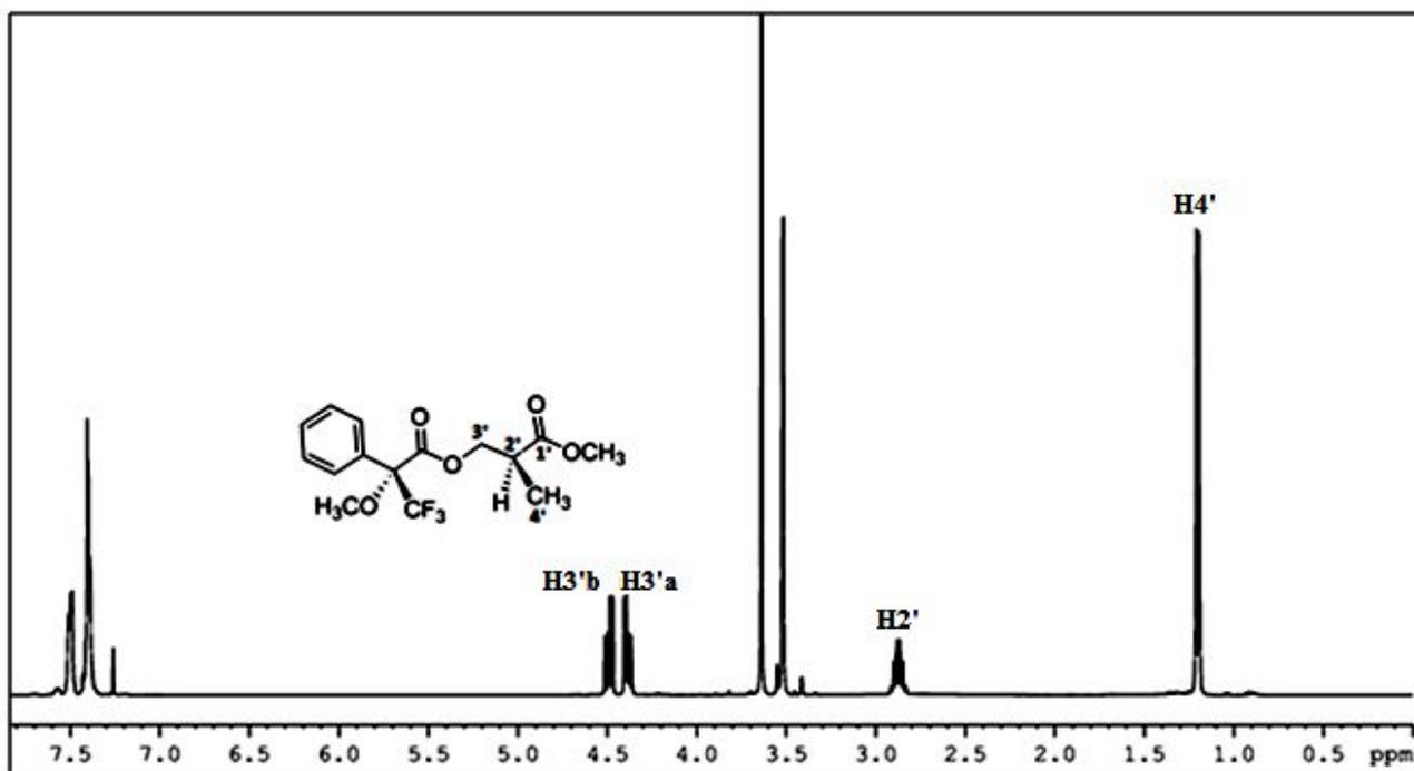
Figure 3.83:  $^1\text{H}$  NMR spectrum of compound Ib (*S/R*-MTPA ester) in  $\text{CDCl}_3$
