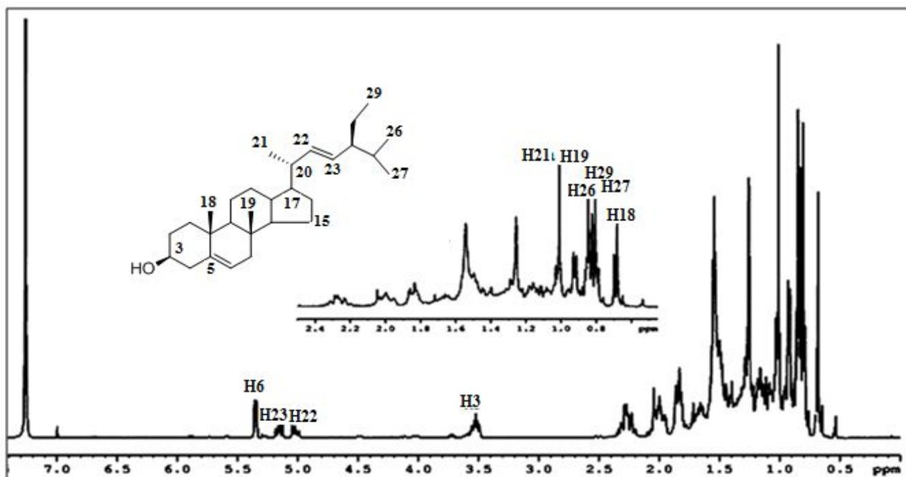
Figure 3.42: <sup>1</sup>H NMR spectrum of compound 304 in CDCl<sub>3</sub>
