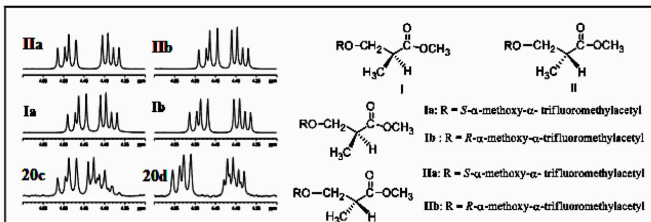
Figure 3.86:  $^1\text{H}$  NMR signals (400 MHz;  $\text{CDCl}_3$ ) due to the methylene protons at C-3 for the compounds **Ia**, **IIa**, **Ib** and **IIb**
